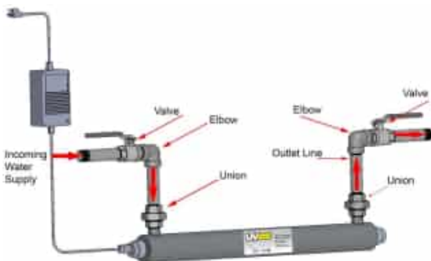
Typical Horizontal Installation
